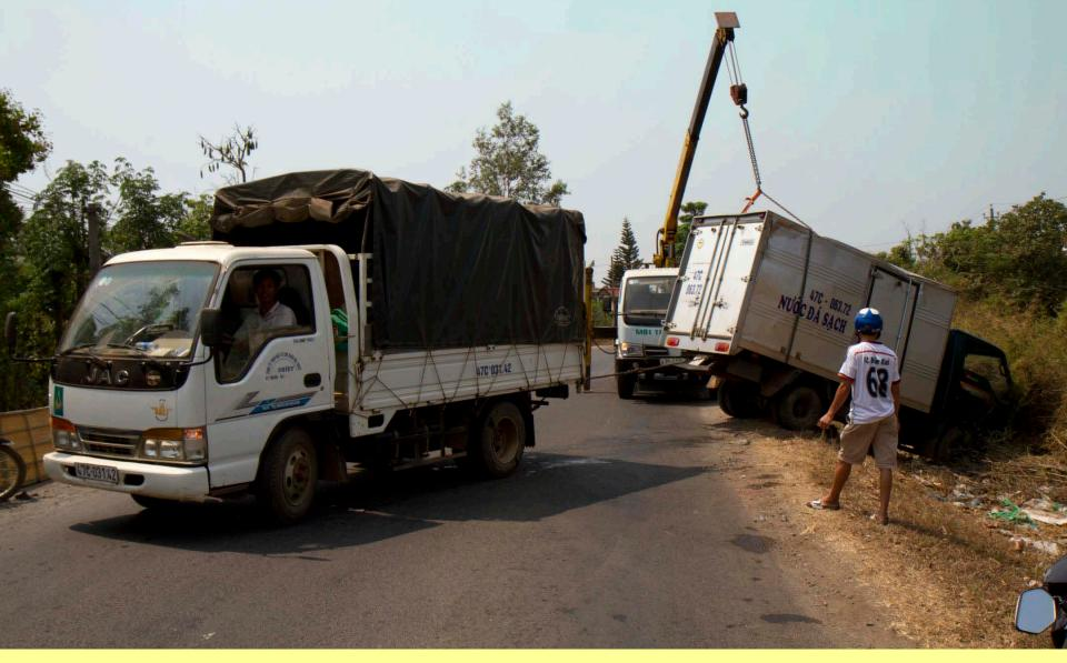
Two rescue trucks needed: lifter and tower. But (a) engine of rescuee must do its bit, (b) rescuee is rear wheel drive, (c) look where the chain is.
